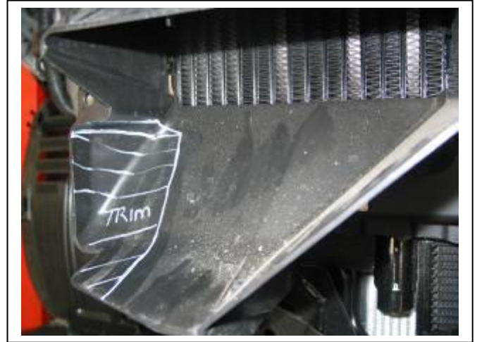
Figure 4: Approximate trim on drivers side shroud
