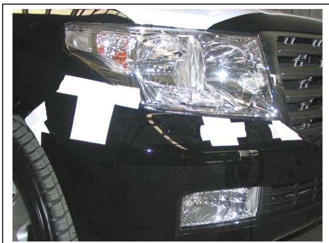
Figure 1: Bumper templates attached. Cut bumper cover removed for photo.
