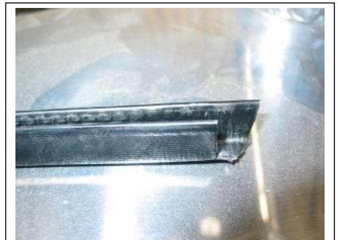
Figure 12: 6mm clip lock trim end trim
