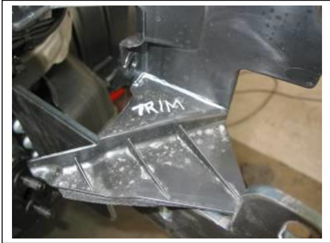
Figure 3: Approximate trim on passengers side shroud
