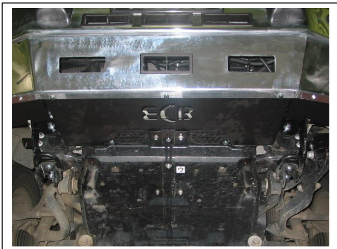
Figure 19: Centre under body guard fitted.
