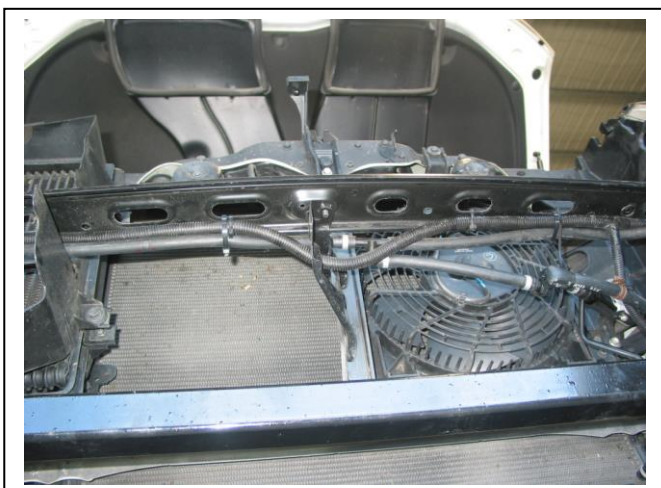
Figure 7: Wiring and headlight washer loome attachment under grille support.
